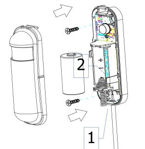
Replace the new battery and install the cover back.
