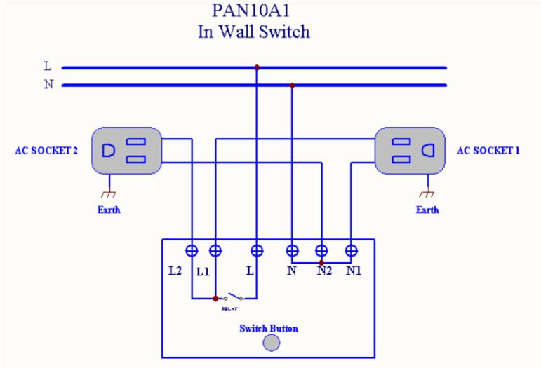
Fig 2. PAN10 Assembling
